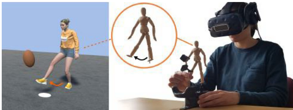
Figure 17: We propose to use a tangible prop to control a human-like avatar during seated virtual experiences. By manipulating the prop, users perform kinematics similar to those of the avatar and experience physical interactions with it. We show that such controllers can enhance the sense of presence and embodiment compared to traditional gamepad controllers.
