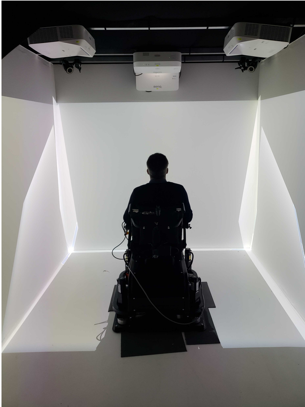
Figure 9: Participant driving in a virtual environment with our simulator
