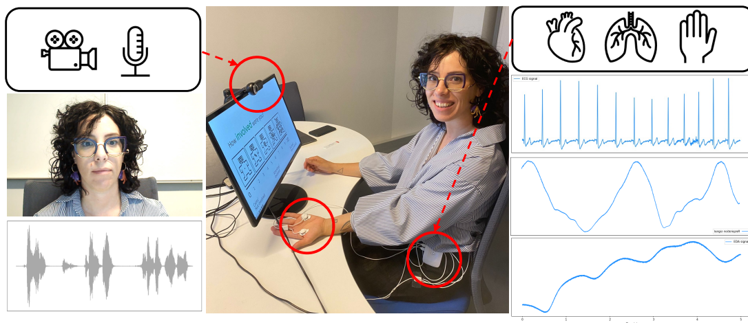
Figure 27: Data collection set-up of StressID.
