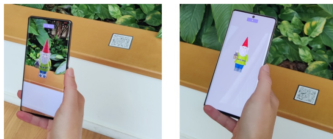
Figure 9: The same stimulus shown in AR (left) and in non-AR (right). In the AR condition, participants were able to move their phone around the virtual object, while in the non-AR condition, they were allowed to rotate the object and zoom with finger gestures.
