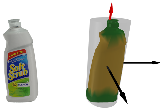
Figure 26: Bleach bottle (left) and a visualization of the corresponding grip selection process (right). Transparent gray volume is the bounding cylinder of the mesh. Red arrow figures the z-axis of the object's frame. The yellow zone illustrates the z-values corresponding to a palmar grip, while the green zone and outwards correspond to a pinch grip.
