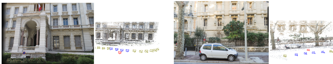
Figure 2: Image-Based Rendering (IBR) techniques use input photographs and approximate 3D to produce new synthetic views.
