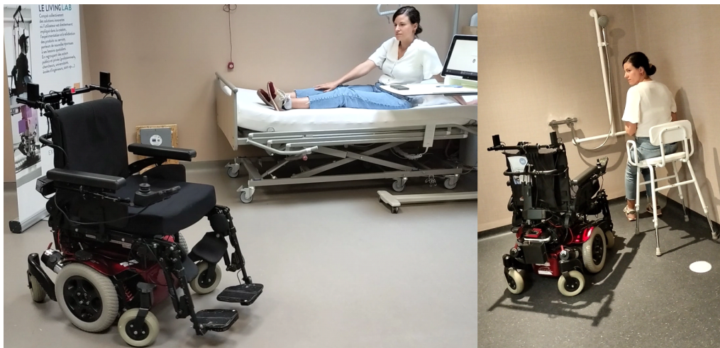
Figure 8: Demonstration of shared control collision avoidance with UWB-based autonomous navigation in narrow environment.
