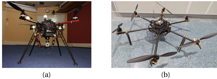
Figure 5: Unmanned Aerial Vehicles Platform. a) one of our customized quadrotors, b) our hexarotor with tilted propellers.
